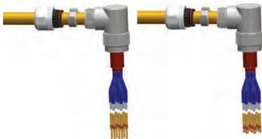
Step 7: Attach contacts to wire leads
