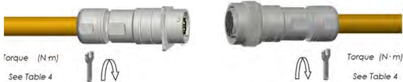
Step 13: Tighten metal nut
