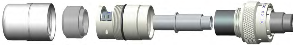
Step 1: Slide components onto cable
