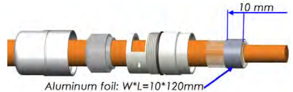
Step 4: Wrap foil over braided shielding
