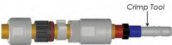
Step 5: Crimp terminal to conductor
