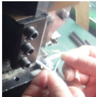
Push crimp contact into opening of crimping machine
